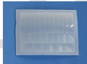
Model: 7708-3 Size: 58*45 Focus: 29.7mm Angle: 80 ° Distance: 14m
